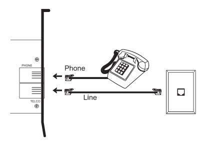
**Figure 4: Connecting Devices**
